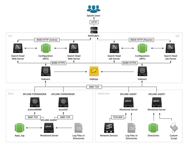
Figure 5. Deployment architecture.
