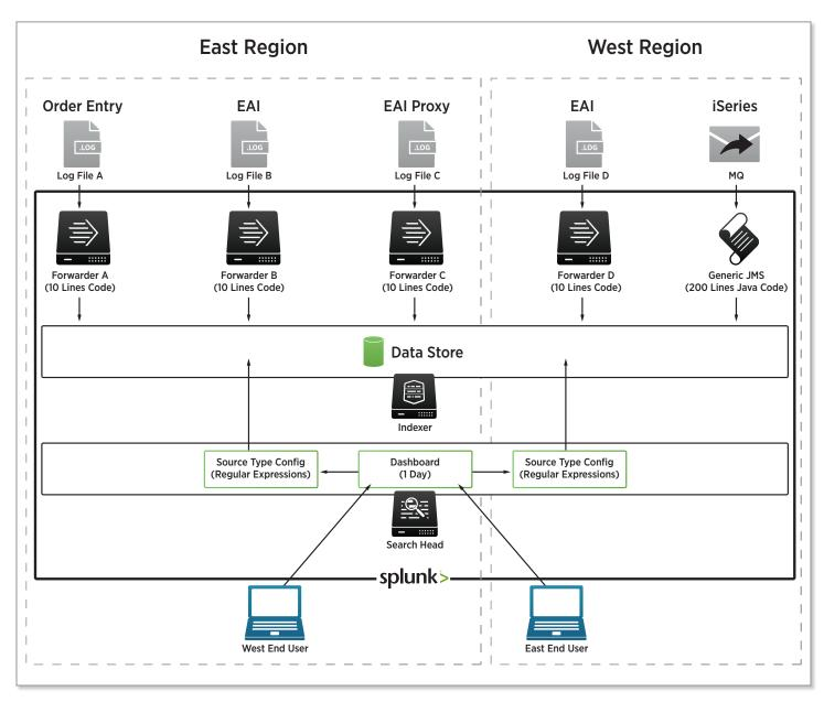
Figure 3. Collecting log data from all systems into Splunk Enterprise.
